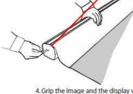
4. Grip the image and the display with your left hand . Remove the locking pin with your right hand. It is now activated!
