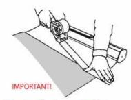
3. Apply packing tape over the joint.
